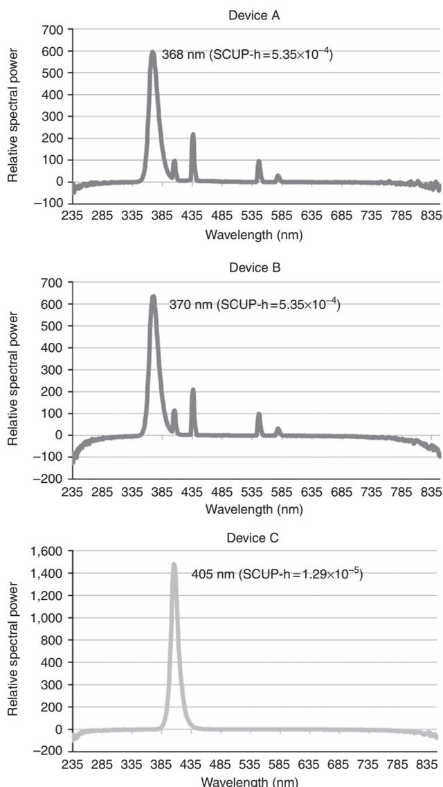
**Figure 1. UV nail lamp spectral power distribution by device.** Note: According to the manufacturer, the negative spectral irradiance values are due to fluctuations in electronic noise, where noise in the dark may be slightly higher than the noise acquired during the sample measurement at a given wavelength. In that case, if there is no signal in the given region, that value appears negative.
